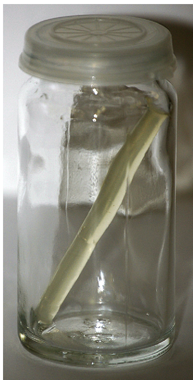
Fig. 7. Hydrogel rod prepared by “click” cross-linking in a syringe followed by extraction of the copper catalysts by 0.1 M aqueous EDTA solution.
